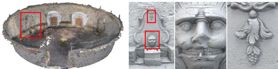
Figure 3: Multi-Scale scene reconstruction. The full, colored mesh (left) and some close-ups (right) with fine details.
