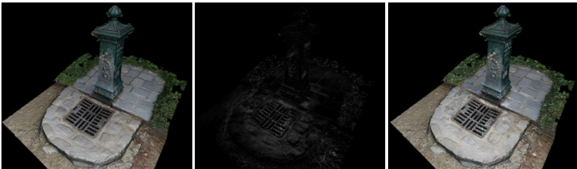
Figure 5. Rendering of the Surface Light Field of a drinking fountain. (Left) Diffuse color. (Center) Residual appearance effects modelled using 16 Hemispherical Harmonics. (Right) Final rendering by combining the diffuse color and the residual appearance effects.
