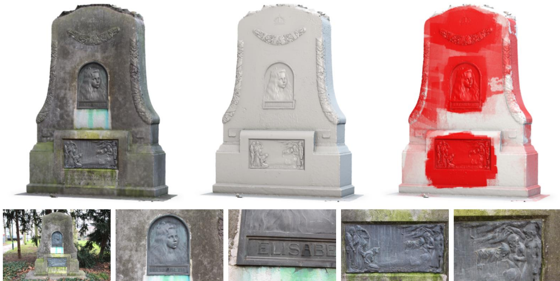
Figure 2. Multi-scale reconstruction of the Elisabeth memorial in color (left), with shading (middle) and false coloring indicating scale (right).
